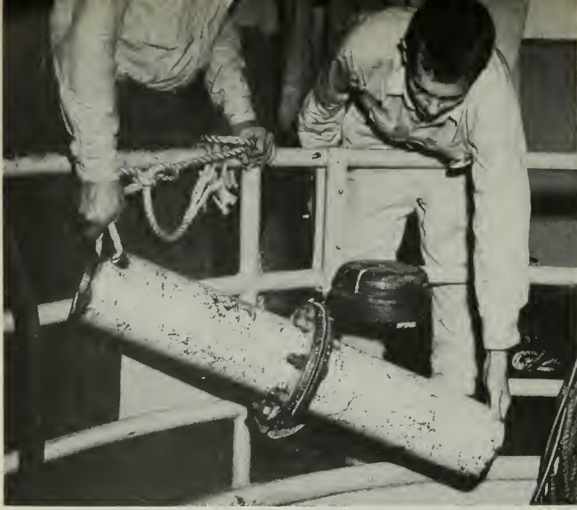
PIPE THIS PROBLEM—Unbolting pipe sections and removing gasket is one of the 'kindergarten' projects used to train divers how to work under water.
